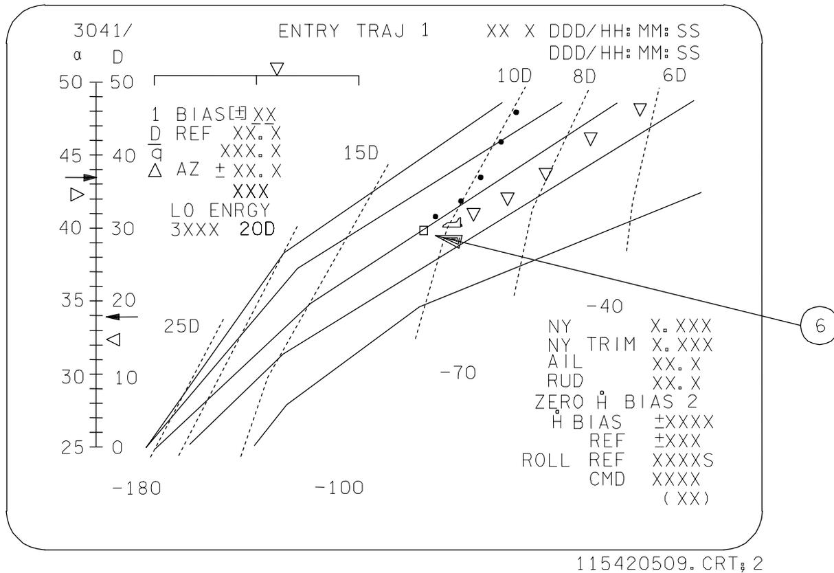
**Figure 5-9. Entry TRAJ 1 (drag less than drag reference)**
