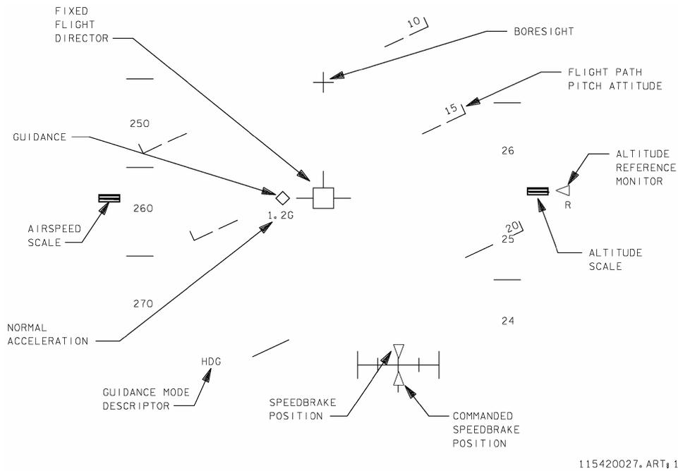
**Figure 5-28. Approach and land display (TAEM heading phase)**
