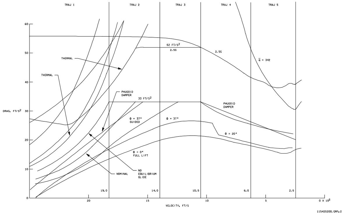
**Figure 5-2. Typical drag versus velocity plot**
